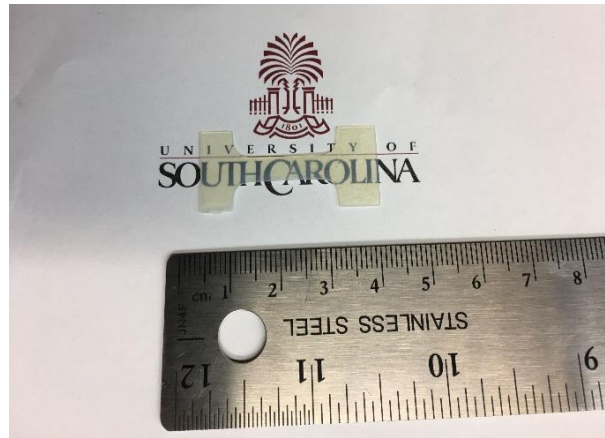
Figure 2.4 Dog-bone shaped film for tensile test
